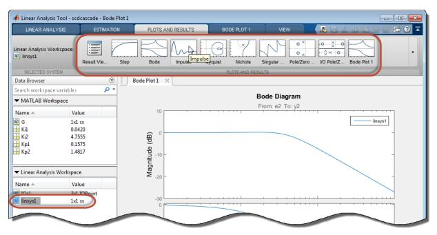
To access the Linear Analysis Tool from a Simulink model, in the Simulink Editor, select **Analysis > Control Design > Linear Analysis**. See the following topics for more information about using Linear Analysis Tool for:
