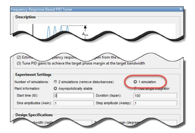
The Frequency Response Based PID Tuner is particularly useful when PID Tuner cannot linearize the plant at the operating point you want to use for tuning. For more information, see Frequency-Response Based Tuning.
