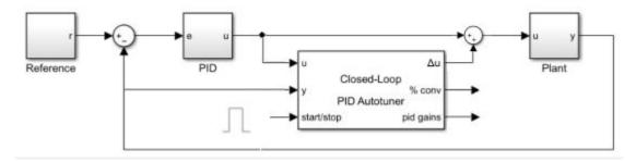
To use the new configuration, in the block parameters, in the **Block** tab, under **Output Signal Configuration**, select **perturbation only**.
